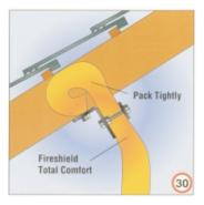
When installing Fireshield Total Comfort transverse to the rafters, a continuous clamping strap should be secured to the underside of each rafter with M6 coach screws or similar.
