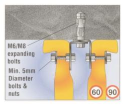
If direct fixing to the concrete soffit is used without the clamping strap, M6 expanding bolts at 300mm centres to the soffit should be used. Adjacent barriers should be wired together. Fireshield Total Comfort should also be draped over the suspended ceiling or wired to the grid. Vertical fixing to a perimeter
