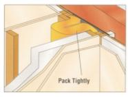
At the junction of a separating and external wall in a timber frame construction, Fireshield Total Comfort should be used to a depth of 300mm to provide a cavity barrier.
