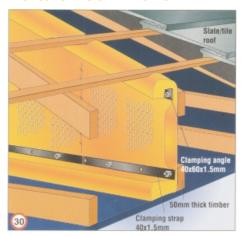
In roof constructions, if the timber is a minimum of 50mm thick, Fireshield Total Comfort needs to be be tightly butt jointed and stitched. The clamping strap should be attached with M6 screws or bolts at a maximum 300mm centres.
