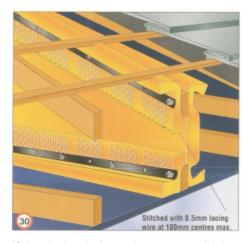
If the timber is less than 50mm thick, both sides of the truss will require the application of Fireshield Total Comfort. In this case, the clamping strap should be attached with screws at a maximum of 400mm centres.
