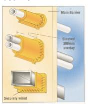
When the area to be treated is penetrated by pipes, ducts or beams, Fireshield Total Comfort should be cut to accommodate the infrastructure and then re-stitched using a minimum 0.5mm wire with a 100mm maximum gap between stitches.
