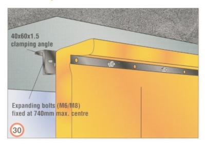
When fixing to a concrete soffit, the continuous clamping angle, size 40x60x1,5mm or 50x50x1.5mm, should be attached with M6 minimum expanding bolts anchored at 740mm maximum centres. 5mm diameter bolts & nuts should be used to attach Fireshield Total Comfort to the clamping strap at maximum 400mm centres.
