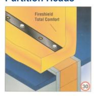
At the head of the fire rated partition, M6 coach screws should be used at a maximum of 400mm centres to attach the clamping strap to the headplate.
