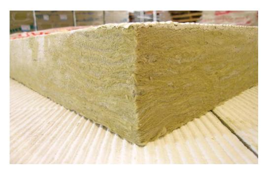
Safire® Raised Access Floor Barriers are purpose manufactured from rock fibre material to seal the void between a raised access floor and the floor slab, thus preventing the spread of fire and smoke within concealed floor spaces and at junctions between floor and walls.
