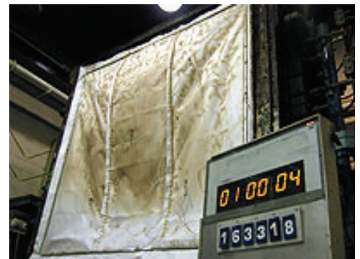
Flamestop FSI undergoing fire test at Bodycote Warrington Fire
