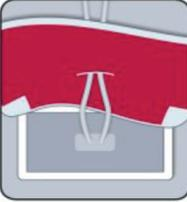
2. Make a slit for the cable and pass the cable through the pad.
