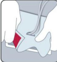
3. Push the pad fully inside the socket box.
